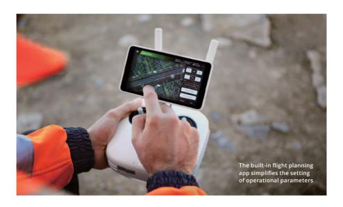
"When setting up the flight path, we need to select the altitude and overlap. The Phantom 4 RTK provides an integrated flight planning app in the remote control including all relevant surveying parameters to make the flight planning easy and efficient," says Philipp Mielke, Teamleader Business Unit Digital Object Survey and UAV at STRABAG.
