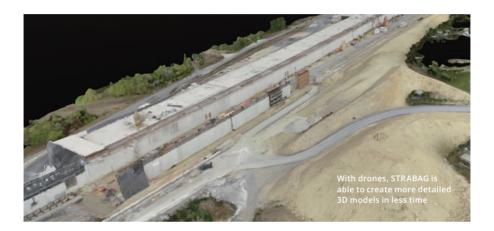
"The use of drones for construction mapping has a lot of advantages. Their integration changes our workflow and simplifies many operational steps. Conventional surveying methods do deliver 3D models as well, but digital terrain models created from drone data provide a higher point density, and therefore reality is portrayed in much higher detail," says Thomas Gröninger, Head of Business Unit Digital Object Survey and UAV at STRABAG.
